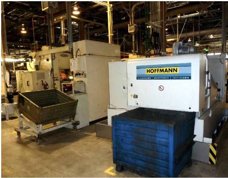
Figure 2: HOFFMANN suction belt filter in the customer's plant
